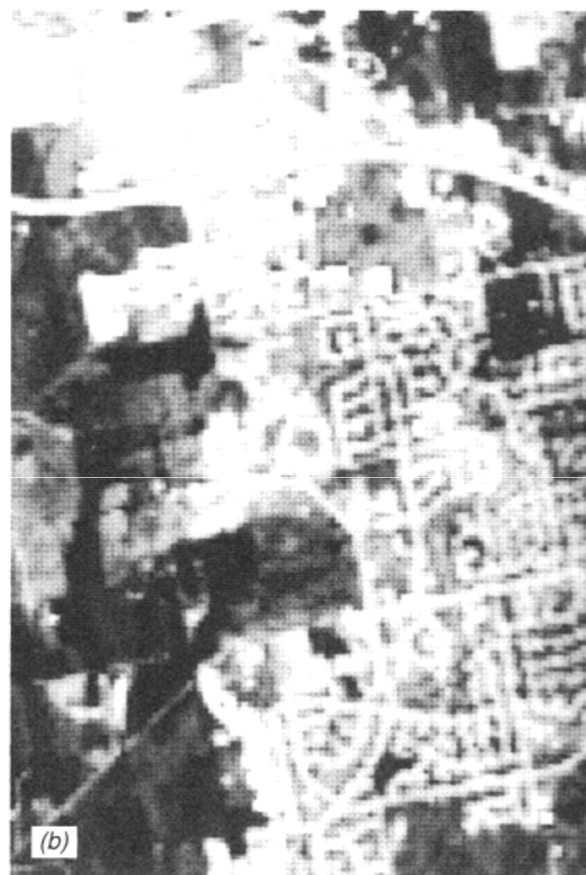
Figure 7.10 Result of applying noise reduction algorithm: (a) original image data with noise-induced “salt-and-pepper” appearance; (b) image resulting from application of algorithm shown in Figure 7.9.
