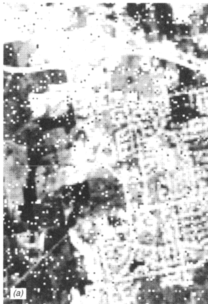
Figure 7.10 Result of applying noise reduction algorithm: (a) original image data with noise-induced “salt-and-pepper” appearance; (b) image resulting from application of algorithm shown in Figure 7.9.
