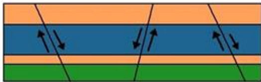
2. Layers are cut by normal faults
